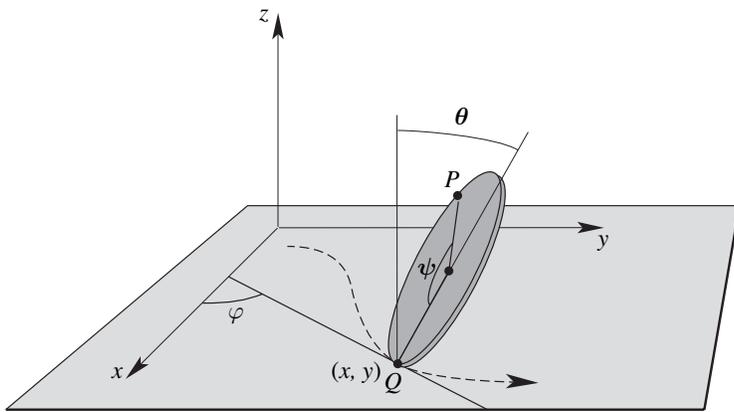
Figure 2. The geometry for the rolling disk.
