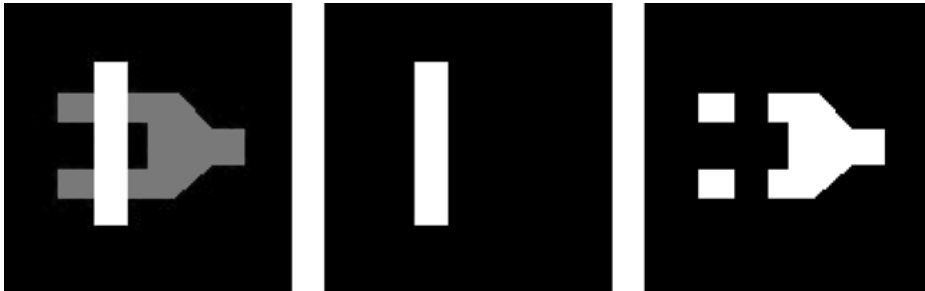
Figure 1. From left to right, these figures are the original image used in the first numerical example and the two regions obtained from it by the preliminary segmentation (without depth) procedure. The resolution of the images is 128 \times 128 .
