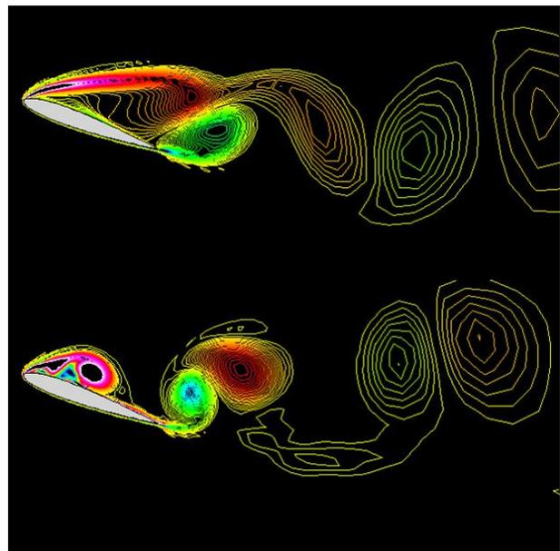
*Figure 7: Flow separation on an airfoil at a high angle of attack can be delayed by periodic blowing and suction through small holes, to reduce drag. Top, uncontrolled; bottom, controlled (S.-C. Huang and J. Kim, UCLA).*
