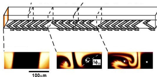
*Figure 2: Pressure-driven flow in a microchannel with small amplitude “herring-bone” grooves on one side leads to a swirling motion and rapid mixing, a precondition for effective use of this technology (Stroock et al., Science, 2002).*
