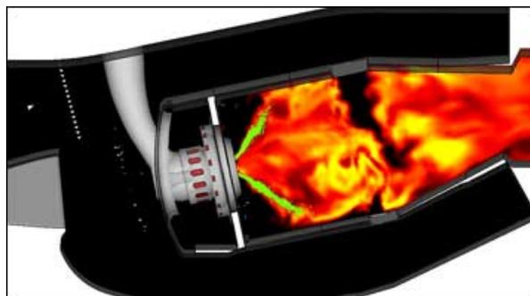
*Figure 6: Computer simulation of a gas-turbine combustor, showing the fuel spray (green) (Stanford University).*
