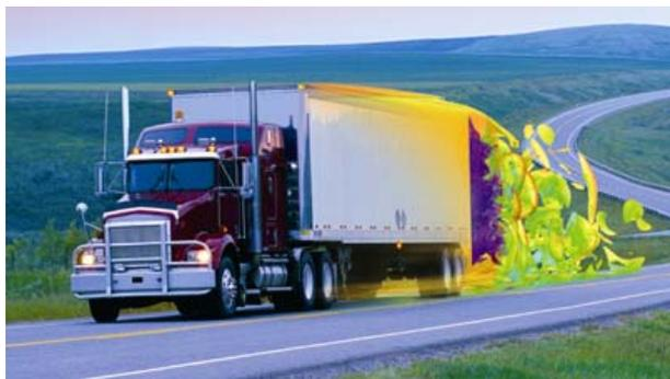
*Figure 5: Computer simulation of the turbulent wake behind a truck (Fluent, Inc.).*
