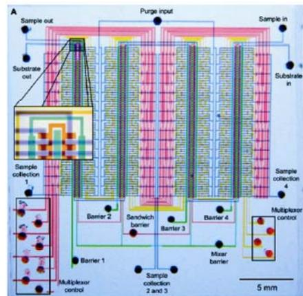
Figure 1: Microfluidic device containing 2056 integrated channels (Thorsen et al., *Science*, 2002). Such devices are revolutionizing biomedical science.
